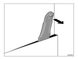
■ After removing the screws from the chimney, slide the lever between chimney and chimney extension and gently apply pressure to ease the chimney from its hooks.
